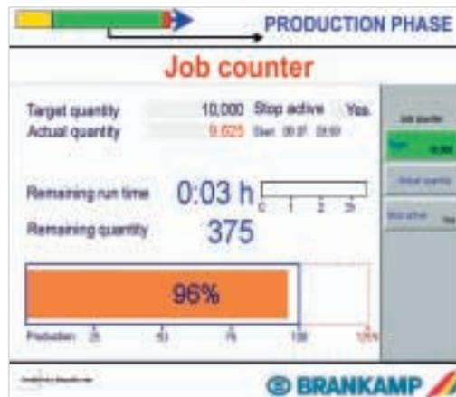
At the same time, the bar graphs are displayed in different colours to distinguish between the individual production phases. Thus, the green graph stands for the current production phase. The length of the bar and the per-
