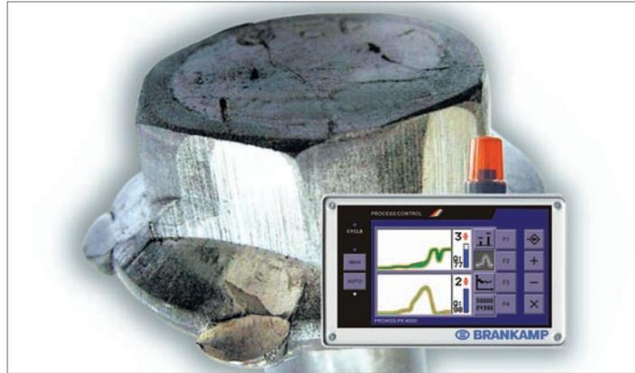
BRANKAMP Rotator monitoring system; screws with "ears" in inset at top right
