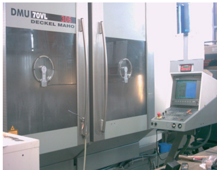
BRANKAMP CMS on a MAHO DMU 70VL. The 5-axis machining centre processes high-precision components. The VL features a twin-table and two machining compartments thereby enabling continuously alternating processing.
