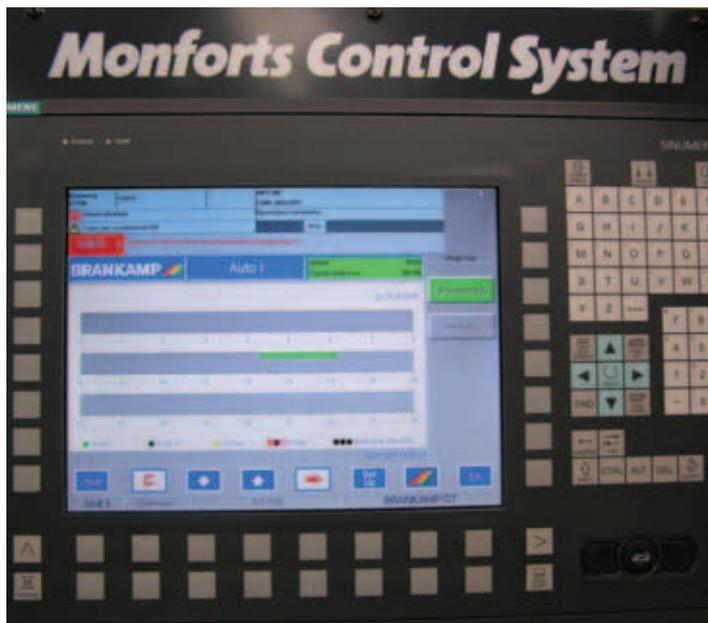
BRANKAMP NC 100 integrated into the controls for a Monfort MCH 500. The NC lathe with a turret for short parts to be turned was equipped with ProcessMonitoring for the Russian market, and it manufactures drive parts for trucks.
