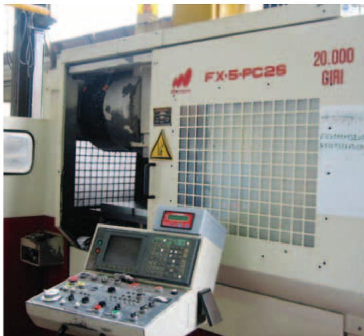
BRANKAMP CMS on a Matsuura FX-5-PC2S. This processing centre is used to manufacture parts for the aircraft industry, such as fuselage parts for the Airbus.
