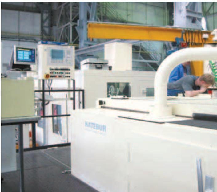
A BRANKAMP PK 6000 on a Hatebur AMP 30 S. This multi-stage press is used to manufacture gearwheel blanks, flange-collar nuts and cam blanks. The Hatebur unit has a total force of pressure of 2,500 kN and weighs 36 tonnes.
