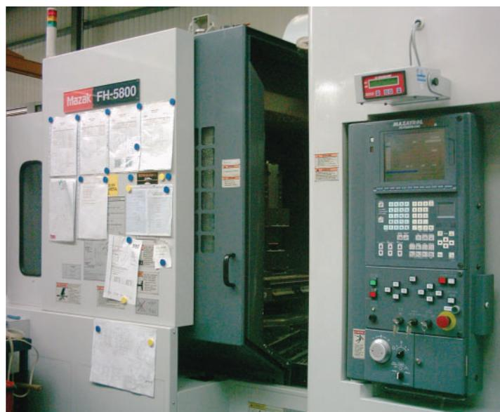
The BRANKAMP CMS ProcessMonitoring system, in use on a horizontal Mazak FH 5800 processing center.
