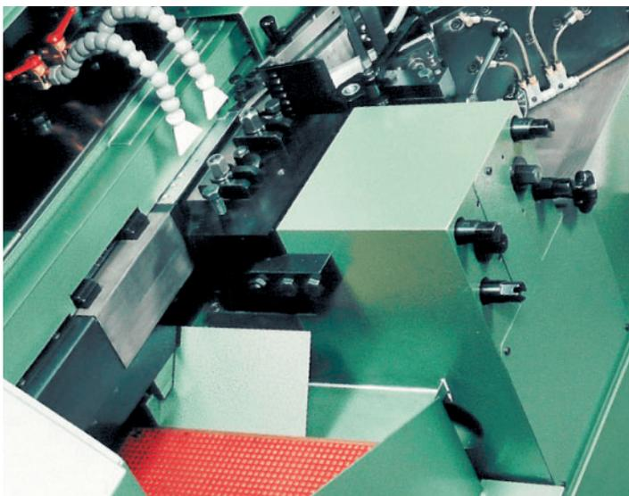
Thread roller with adjustment screw
