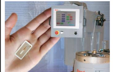
In modern manufacturing, every centimeter of space is used. The BRANKAMP ET 500 – the innovative front-end system of the ECO 500 – takes this into account: the operating terminal and the engineering are separated from one another. It is only the small ET industrial terminal which needs to be machine-mounted.
