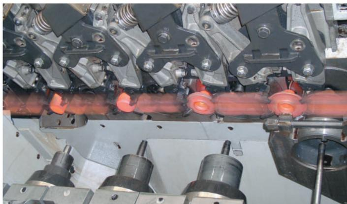
Production underway: the automated multi-stage press from Hatebur
