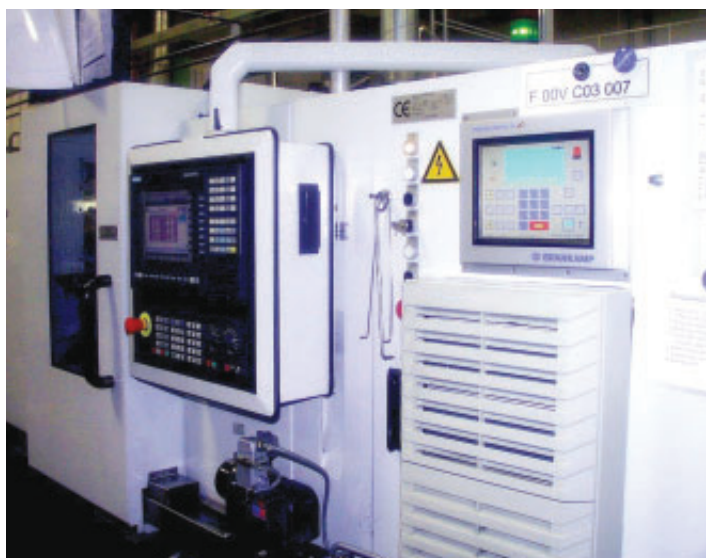
A BRANKAMP C100 on an AG200 belonging to the Schütte company. The auto parts supplier Bosch produces injector bodies for fuel injection on the multiple drill.
