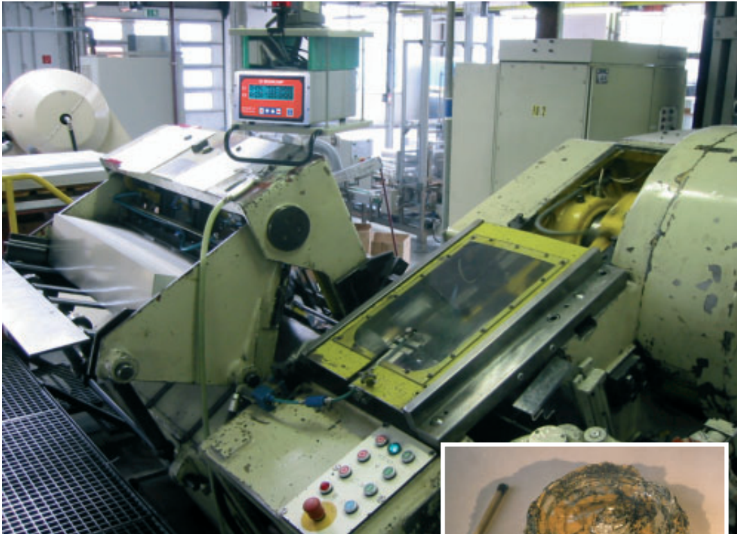
BRANKAMP B100: Defective parts are immediately recognized and sorted out.
