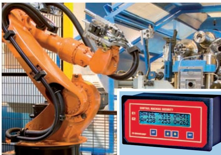
BRANKAMP ProcessMonitoring systems are also increasingly being used on robots and handling units. In our example, they are monitoring a welding robot which manufactures for the automotive industry. The systems have already proven their worth in a large number of other applications in manufacturing practice.
