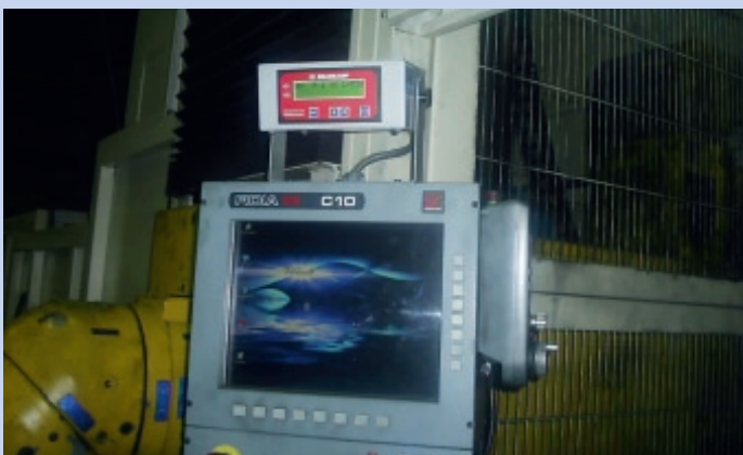
A BRANKAMP CMS in use on an Auerbach bed-type milling machine, type IA 5B. The powerful milling machine has a pivoting HSC spindle and is suited to many types of metal processing.
