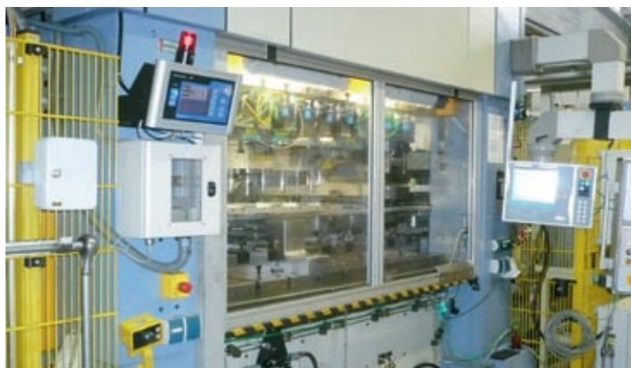
BRANKAMP PK4U with sorting function installed on Helmerding-press
