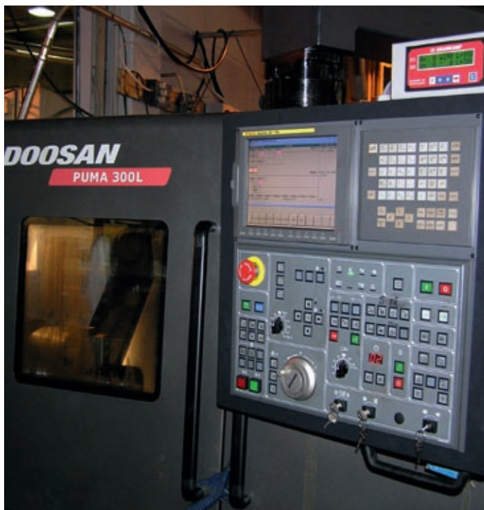
A BRANKAMP CMS-System installed on a Doosan Puma 300L.
